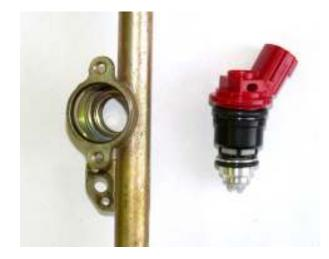
Step 3: Install the lower injector adapter. This is done by pushing the injector into the lower injector adapter.
