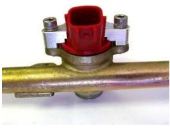
Step 5: Use an allen wrench to tighten the injector cap to the fuel rail and admire your finished product.
