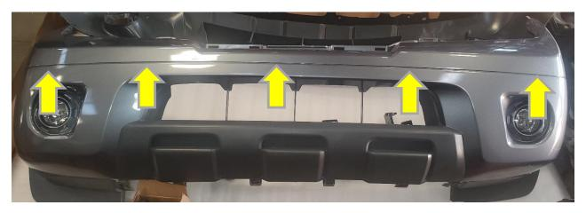
Note: If trimming bumper fascia on truck, ensure to protect AC condenser, AC lines and any exposed wiring from damage.
