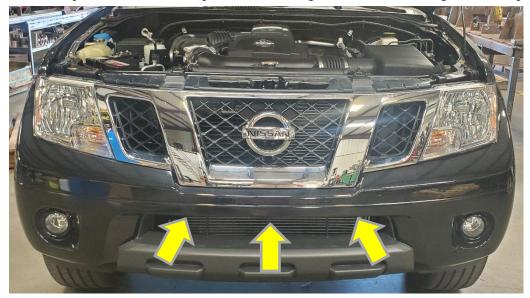
7. Trim bumper fascia and inner supports along the trim line as show in the picture. Cover the bumper with blue tape to avoid any scratches. A cut off wheel on an angle grinder works well for this.
