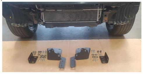
3. Attach lower frame mounts to frame mounts with the head of the bolt to the inside of the truck BEFORE installing the frame mount to the frame horns. Leave all hardware hand tight. Make sure to use washers and lock washers on the lower mounts.
