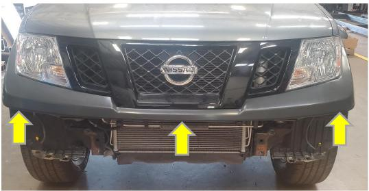
9. Remove 4 bolts with a 17mm socket front bumper support and removed bumper support. Set bolts aside to be reused. (Picture shows one side)
