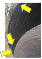
2. Unplug fog lights from both sides by reaching inside the inner fender.
