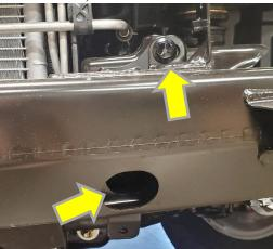
10. Remove 2 bolts with a 17mm socket from tow hook and remove tow hook. Set bolts aside to be reused.
