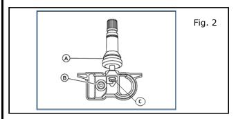
8) a) Unscrew Torx bolt (C) using Torx #10 socket/bit. See Fig. 2.
