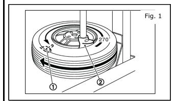
7) Carefully lift tire onto turn-table and position valve hole (and tire pressure sensor) 270° from mounting/dismounting head (2). See Fig. 1.
