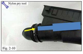
(j) On a workbench, use a nylon pry tool to raise the area around the locating tab to remove the OE air inlet duct from the lower air box (Fig. 2-10).
