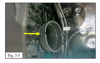
(f) At the vehicle, install the TRD air horn into the inner fender. Make sure that the slot is to the top (Fig. 3-5).
