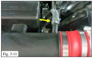
(l) Connect the crankcase vent hose to the inlet tube and secure it with the spring clamp over the intake tube nipple (Fig. 3-11).
