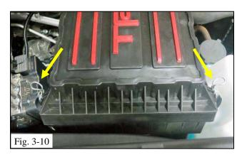
(k) Engage the clips to secure the air box lid into place (Fig. 3-10).
