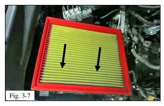
(h) Install the TRD air filter in the lower air box housing (Fig. 3-7).
