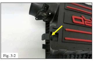
(c) Install the sensor harness clip, removed in Step 2(k) (refer to Fig. 2-11), into the TRD upper air box (Fig. 3-2).
