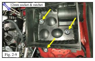
(i) Remove the three M8 bolts holding the lower air box and remove it (Fig. 2-9).
