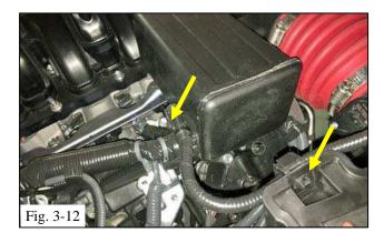
(m) Attach the mass airflow wire harness to the side of the TRD resonance chamber (left arrow, Fig. 3-12) and to the top of the TRD upper air box (right arrow, Fig. 3-12).
