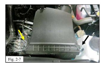
(g) Unclip the two retaining clips on the air box lid and remove the complete assembly (Fig. 2-7).
