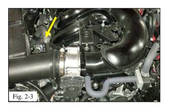
(c) Squeeze the clamp on the PCV hose, slide it back and disconnect the hose from the inlet duct (Fig. 2-3).
