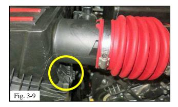
(j) Make sure the two tabs on the air box lid and lower housing are fully engaged (Fig. 3-9).
