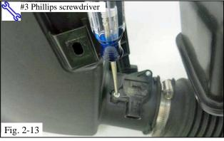
(m)Remove the two screws and remove the mass airflow sensor from the OE air box lid (Fig. 2-13). Keep the screws and sensor for reuse.
