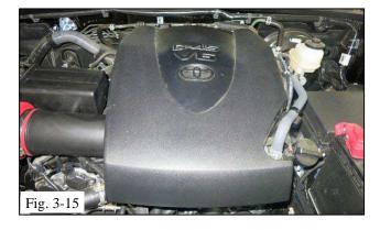
(p) Reinstall the engine cover (Fig. 3-15).
