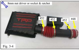
(e) Assemble the bellows, inlet tube and coupler, then connect the coupler to the upper air box. Tighten the #52 hose clamps only at this time (Fig. 3-4).
