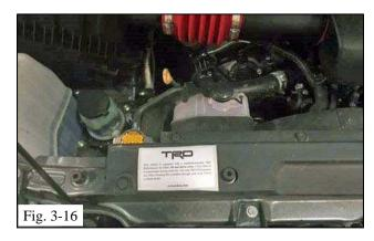
(q) Apply the reusable filter notification label to the radiator support cover on the passenger side, opposite the oil type label (Fig. 3-16).
