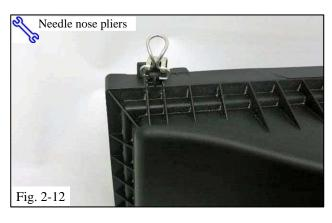
(1) Remove the air box retaining clips and retain them for reuse (Fig. 2-12).
