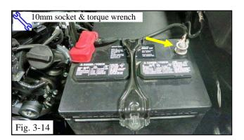
(o) Reconnect the negative battery cable to the negative battery terminal (Fig. 3-14).
