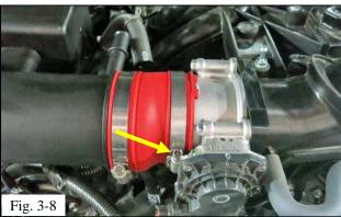
(i) Push the coupler end of the the assembled TRD intake system over the throttle body, then tighten the #48 hose clamp (Fig. 3-8).
