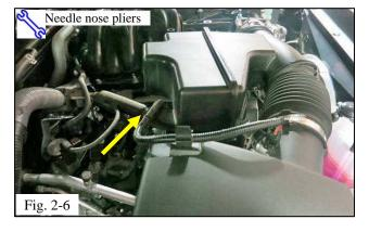
(f) Unclip the sensor wiring harness from the side of the factory resonance chamber (Fig. 2-6).
