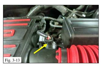
(n) Plug in the mass airflow sensor connector (Fig. 3-13).
