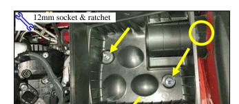
(g) Reinstall the lower air box housing with the three M8 bolts removed in Step 2(i). Make sure to align the tang on the lower air box with the slot in the air horn (Fig. 3-6).
