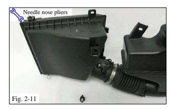
(k) Unclip the sensor wiring harness clip from the top of the OE air box lid and retain it for reuse (Fig. 2-11).
