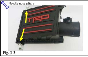
(d) Install the air box retaining clips, removed in Step 2(l) (refer to Fig. 2-12), into the TRD upper airbox (Fig. 3-3).
