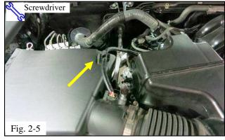
(e) Unclip the sensor wiring harness from the top of the air box lid (Fig. 2-5).
