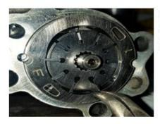
Remove c-clip on the shaft and use needle nose pliers to remove impeller vanes.
