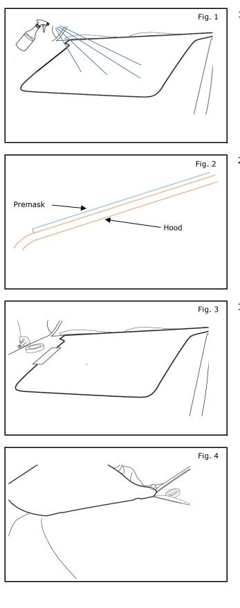
1) Using a clean lint free micro fiber cloth clean surface of hood with 90% or greater isopropyl alcohol. Allow area to dry completely (Fig 1.)
