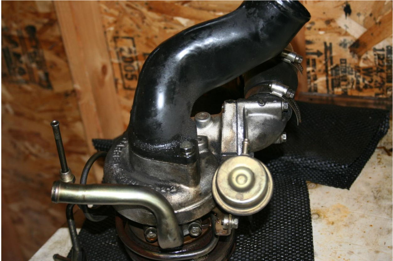
As-removed turbo assembly with inlet pipe, outlet pipe, oil drain pipe, wastegate, etc
