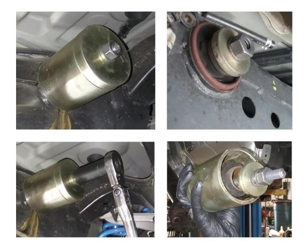
6. <u>Remove Outer Sleeve of Bushing</u>: Align machined pocket of Housing against lip at front-side of Sub-frame. Insert 3/4"ACME Rod through Washer, Housing, and Bushing. Slide <u>Large Plate</u> over ACME Rod at backside of Sub-frame. Lock Assembly into place with 3/4" ACME Nut at each end. Tighten ACME Nuts against each other until Outer Sleeve separates from Sub-frame.
