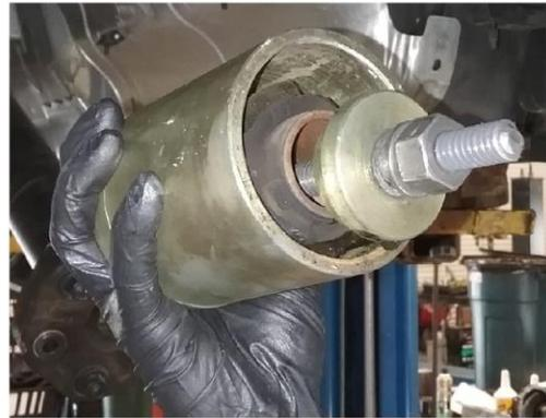
6. **Remove Outer Sleeve of Bushing:** Align machined pocket of Housing against lip at front-side of Sub-frame. Insert 3/4" ACME Rod through Washer, Housing, and Bushing. Slide **Large Plate** over ACME Rod at backside of Sub-frame. Lock Assembly into place with 3/4" ACME Nut at each end. Tighten ACME Nuts against each other until Outer Sleeve separates from Sub-frame.
