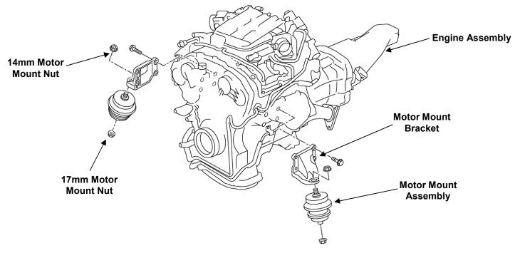
5) Once the motor has been reinstalled onto the engine's cross member, torque the lower nut to between 68 ft/lbs. Again, it is recommended that some form of thread locking compound be applied for additional security.
