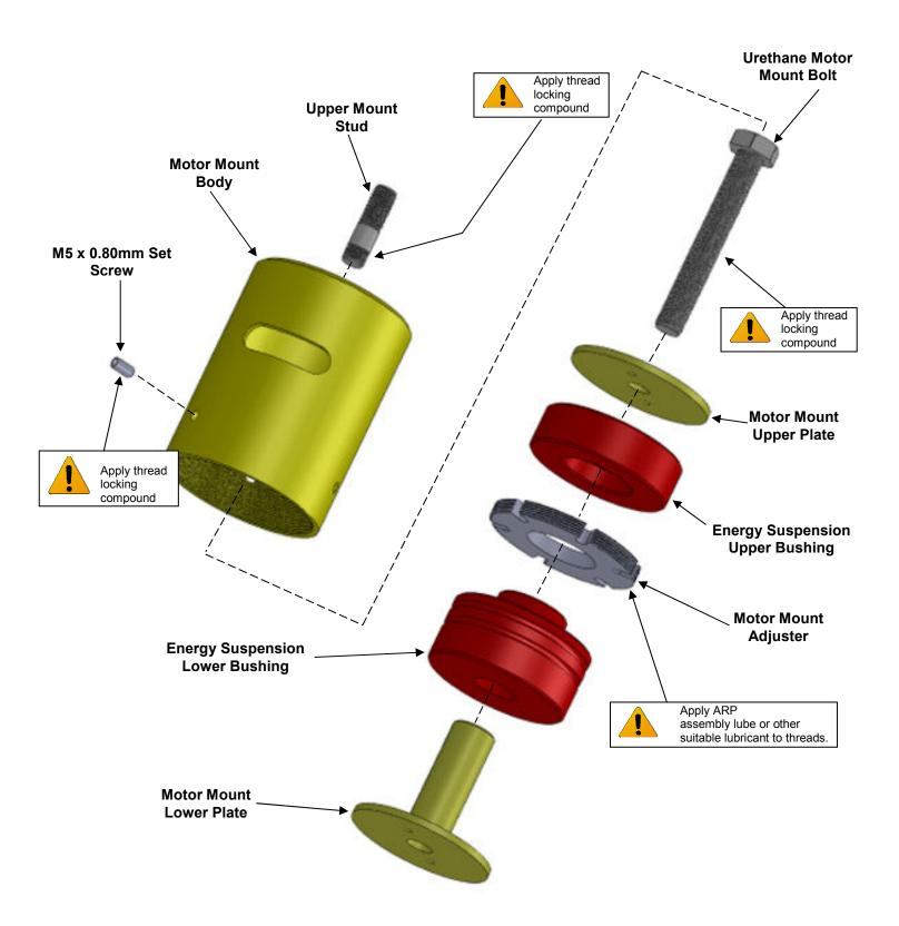
When servicing or adjusting the Z1 Motorsports Urethane Motor Mount Bushings, follow below mentioned steps in sequence when disassembling or reassembling the units. (Refer to the Motor Mount exploded view on the previous page for part sequencing and locations).
