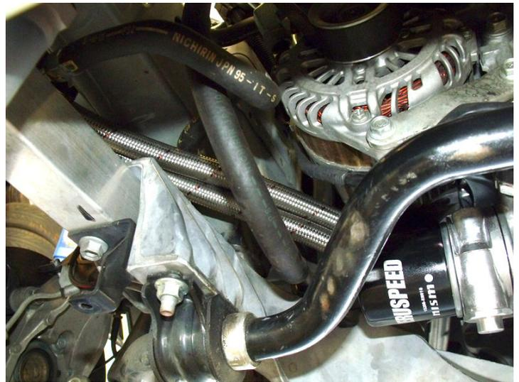
14. If you are planning on changing the engine oil during the installation of the Z1 Motorsports Oil Cooler Kit, remove Engine Oil Drain Plug and drain the engine oil. If you are not planning on performing this step, continue to STEP #16.
