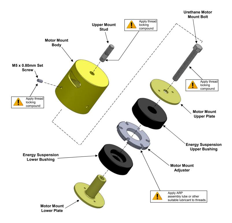
When servicing or adjusting the Z1 Motorsports 300zx Urethane Motor Mount Bushings, follow below mentioned steps in sequence when disassembling or reassembling the units. (Refer to the Motor Mount exploded view on the previous page for part sequencing and locations).
