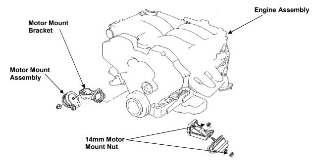
5) Once the motor has been reinstalled onto the engine's cross member, torque the lower nut to between 32 – 44 ft/lbs. Again, it is recommended that some form of thread locking compound be applied for additional security.
