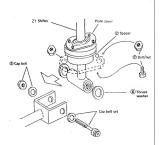
provided bolt and then install the change rod. In this case, remove the tape covering the shifter before installing the change rod.
