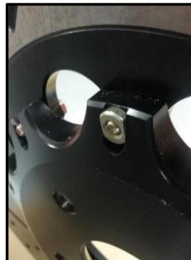
4. Locate M6-1.0 x 20mm bolts. Apply a small amount of Loctite #271 thread locker to the end of each bolt.
