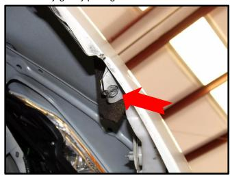
9. Gripping the sides of fascia (circled below) pull the fascia towards you. This part of the fascia snaps in place and will pop loose when a limited amount of force is applied. Once free, carefully remove the fascia from the chassis and set aside.
