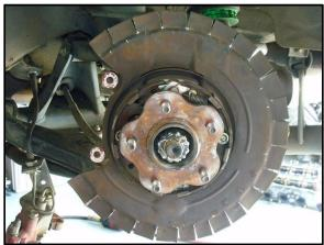
7. Locate the two Z1 Motorsports 300ZX Big Brake Kit Rear Brake Caliper Adapter Brackets and the Stock Brake Caliper bolts removed in Step #5B.
