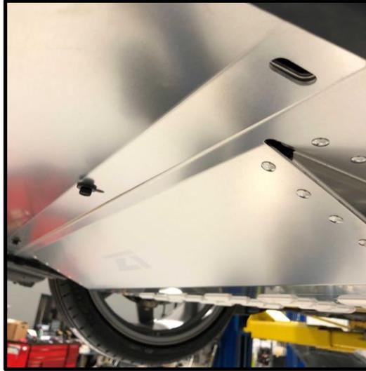
7. Place a nylon spacer above the other middle mounting hole (circled above) between the undershroud panels and the vehicle. Secure with (1) 35mm bolt.
