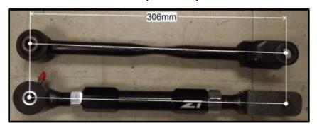
Refer to the alignment chart below for approximate camber at a given length. Z1 recommends professional alignment immediately after installation.
