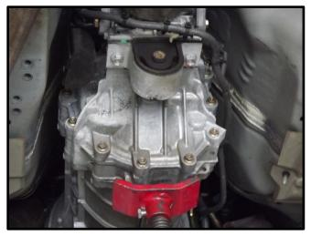
Using the below diagram as a parts guide, refer to this image for part reference in order to complete the removal of the OEM transmission mount as well as to install the Z1 Motorsports Urethane Transmission Mount.
