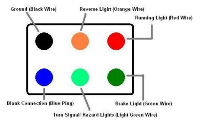
**Warning!** Do Not Connect the Z1 Reverse Fog Lamp Wiring Harness to the Tail Light's Harness. Connect the wires to the harness located on the body! Future removal of the tail lights will be affected.
