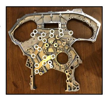
Note: Assure all surfaces and gaskets are clean and dry. Do Not use RTV with these gaskets.
