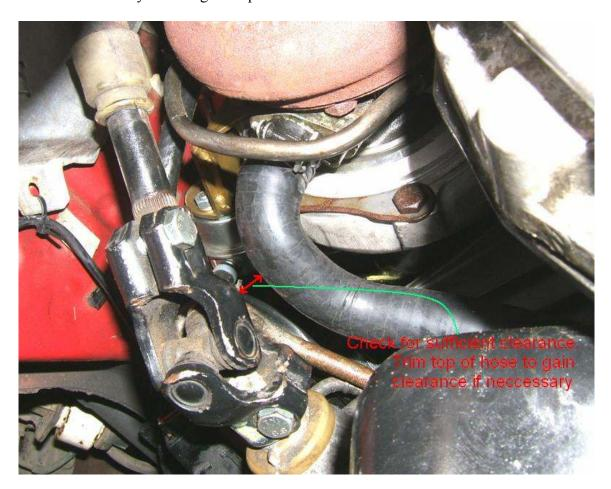
Some applications, particularly those with aftermarket exhaust manifolds, may result in interference between the right side silicone hose and the oil pressure sending unit. We have included a threaded 90 degree adapter fitting included with each kit to relocate the oil pressure sending unit if necessary.
