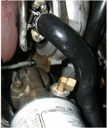
Screw the oil pressure sending unit back into the elbow and plug it back up.
