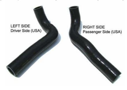
Check for sufficient clearance between the steering knuckle and return hose. Clearance can be increased by trimming the top end of the silicone return hose.
